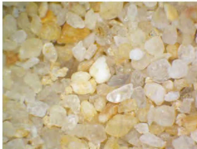
Plate 6: Typical micro appearance of the 600 - 300 micron sand fraction - 6mm field of view.
