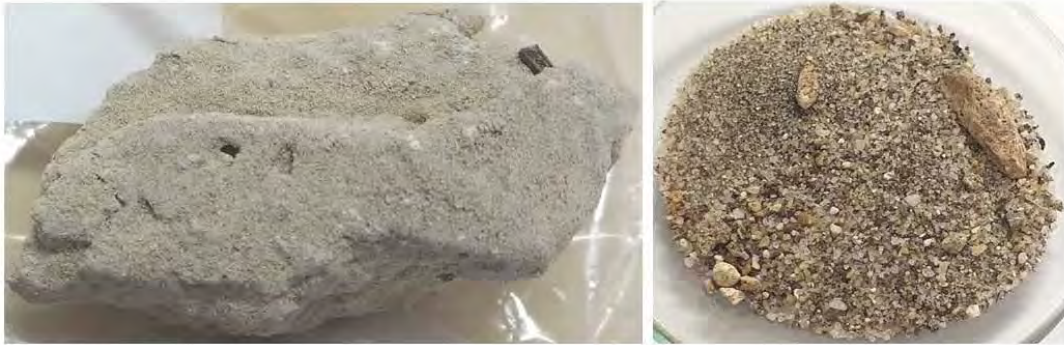
Plate 7: Typical macro appearance of the whole plaster sample and bulk sand fraction (right).
