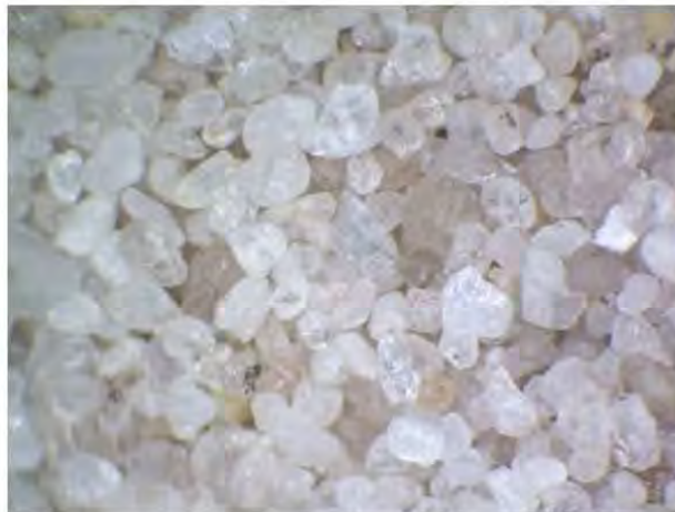
Plate 12: Typical micro appearance of the 600 – 300 micron sand fraction - 6mm field of view.
