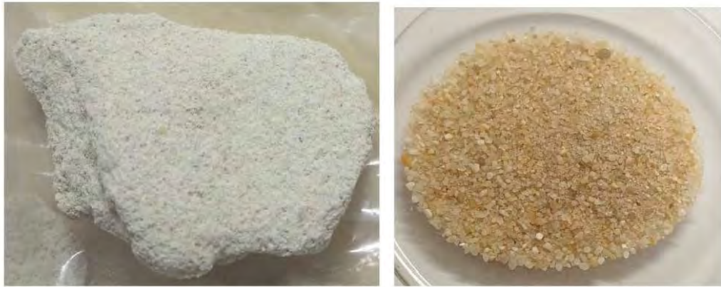
Plate 3: Typical macro appearance of the whole mortar sample (left) and bulk sand fraction (right).
