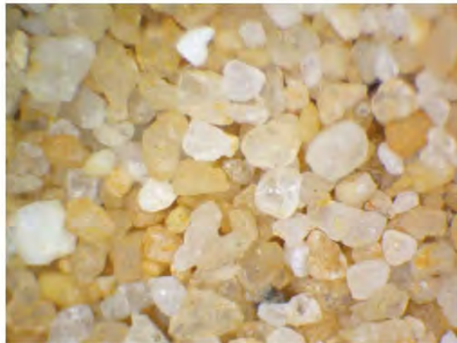
Plate 10: Typical micro appearance of the 600 – 300 micron sand fraction - 6mm field of view.
