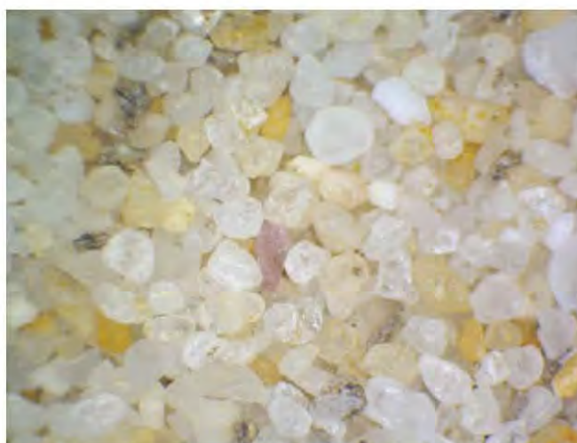
Plate 2: Typical micro appearance of the 600 - 300 micron sand fraction - 6mm field of view.
