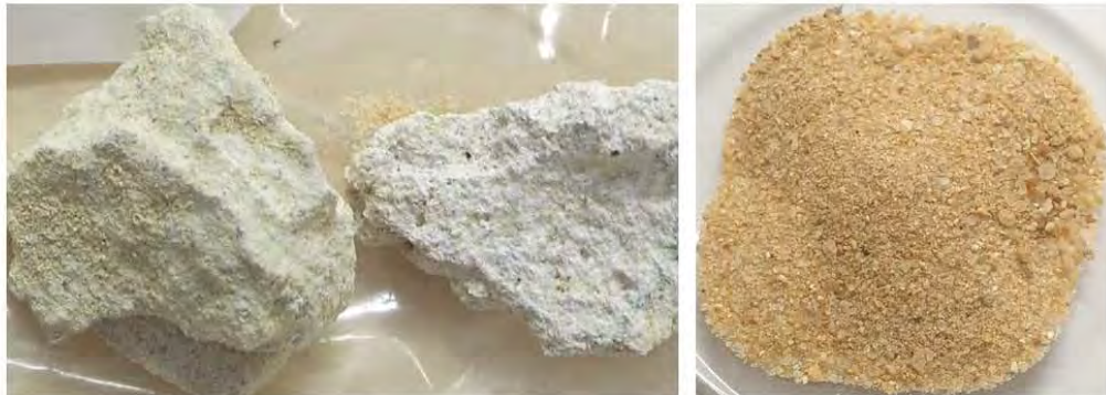
Plate 5: Typical macro appearance of the whole mortar sample and bulk sand fraction (right).
