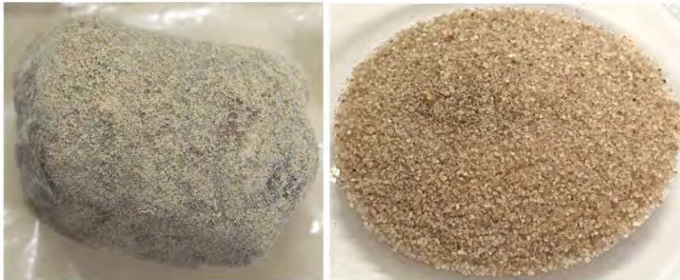
Plate 11: Typical macro appearance of the whole plaster sample and bulk sand fraction (right).
