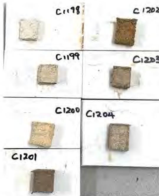
Plate 15: Compacted and dried samples from the original mortar mixtures
