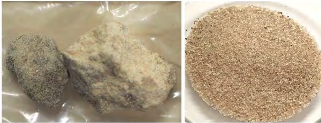
Plate 13: Typical macro appearance of the whole plaster sample and bulk sand fraction (right).
