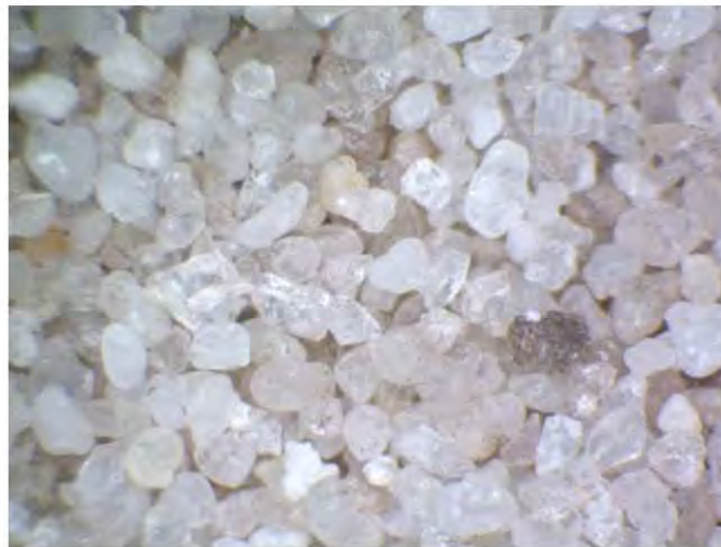
Plate 14: Typical micro appearance of the 600 – 300 micron sand fraction - 6mm field of view.
