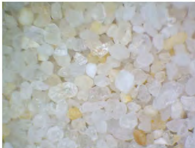
Plate 4: Typical micro appearance of the 600 - 300 micron sand fraction - 6mm field of view.
