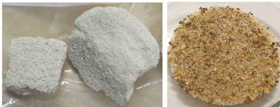
Plate 1: Typical macro appearance of the whole mortar sample (left) and bulk sand fraction (right).
