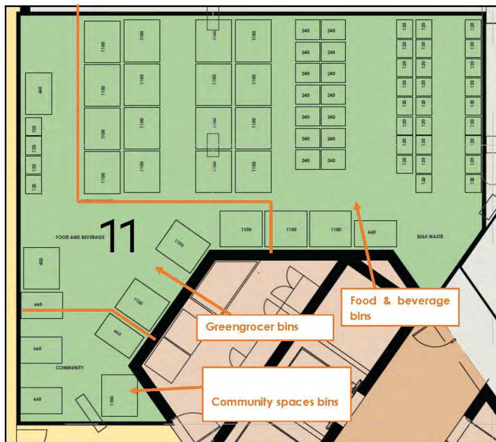
Figure 5: Commercial bin store
