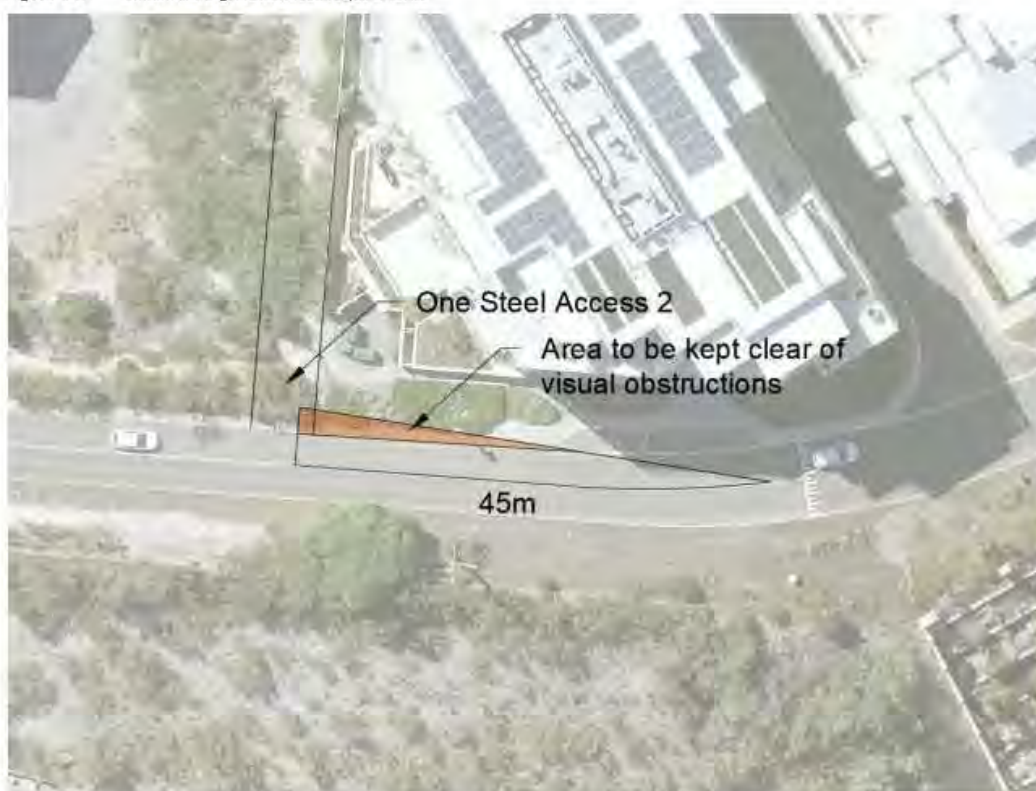
Figure 4-2 Minimum Sight Distance Requirements
