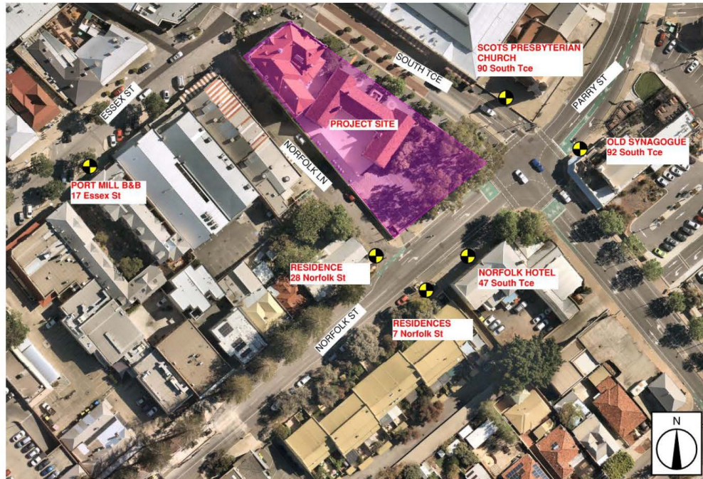
Figure 4: Attended Noise Monitoring Locations
