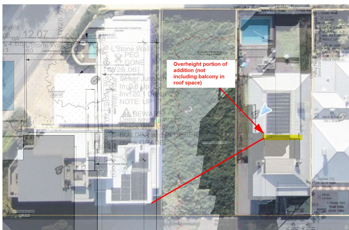
Figure 5: Transition from 4 Rule Street (left part of image) to subject site, noting predominant bulk impact of the former is located substantially closer to the street than that of the latter.
