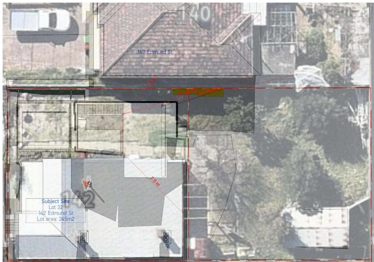
Figure 2: Impact of roof deck to northern neighbours back yard.
