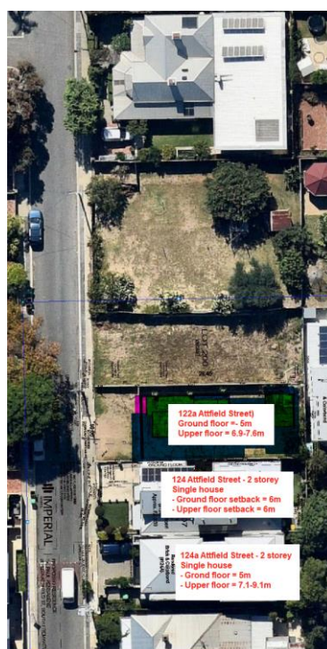
Figure 1: Prevailing streetscape including the ground and upper floor setbacks of the adjoining southern two Single houses.
