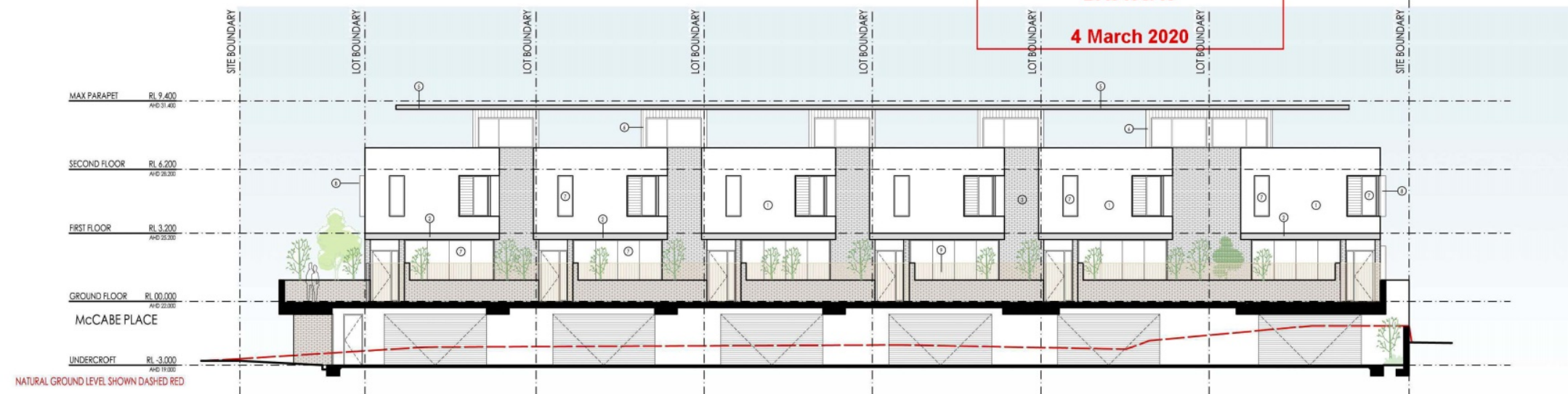
SECTION BB (NORTH ELEVATION OF SOUTH LOTS 6-11) 1: 200
