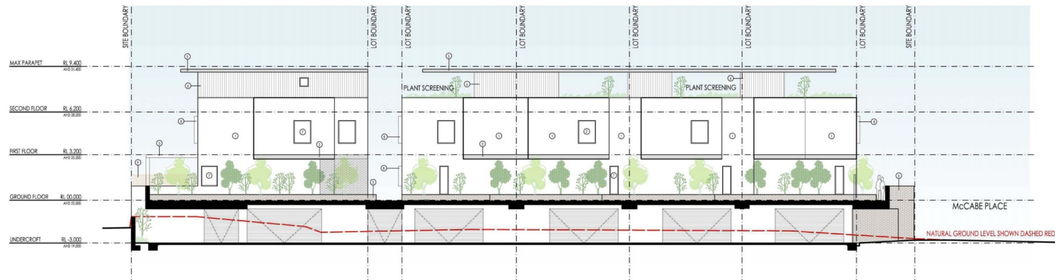
SECTION AA (SOUTH ELEVATION OF NORTH LOTS 1-5) 1: 200
