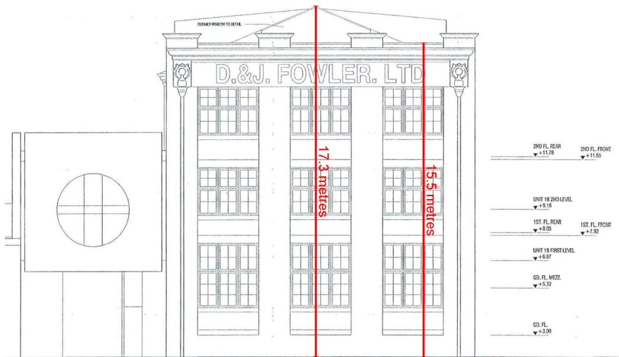
Figure 6 – Pakenham Street (east) elevation of the mixed use development at 33-35 Pakenham Street (D & J Fowler Building) north of the subject site. Note: Maximum building height of 15.5m (parapet) to 17.3m (roof ridge).
