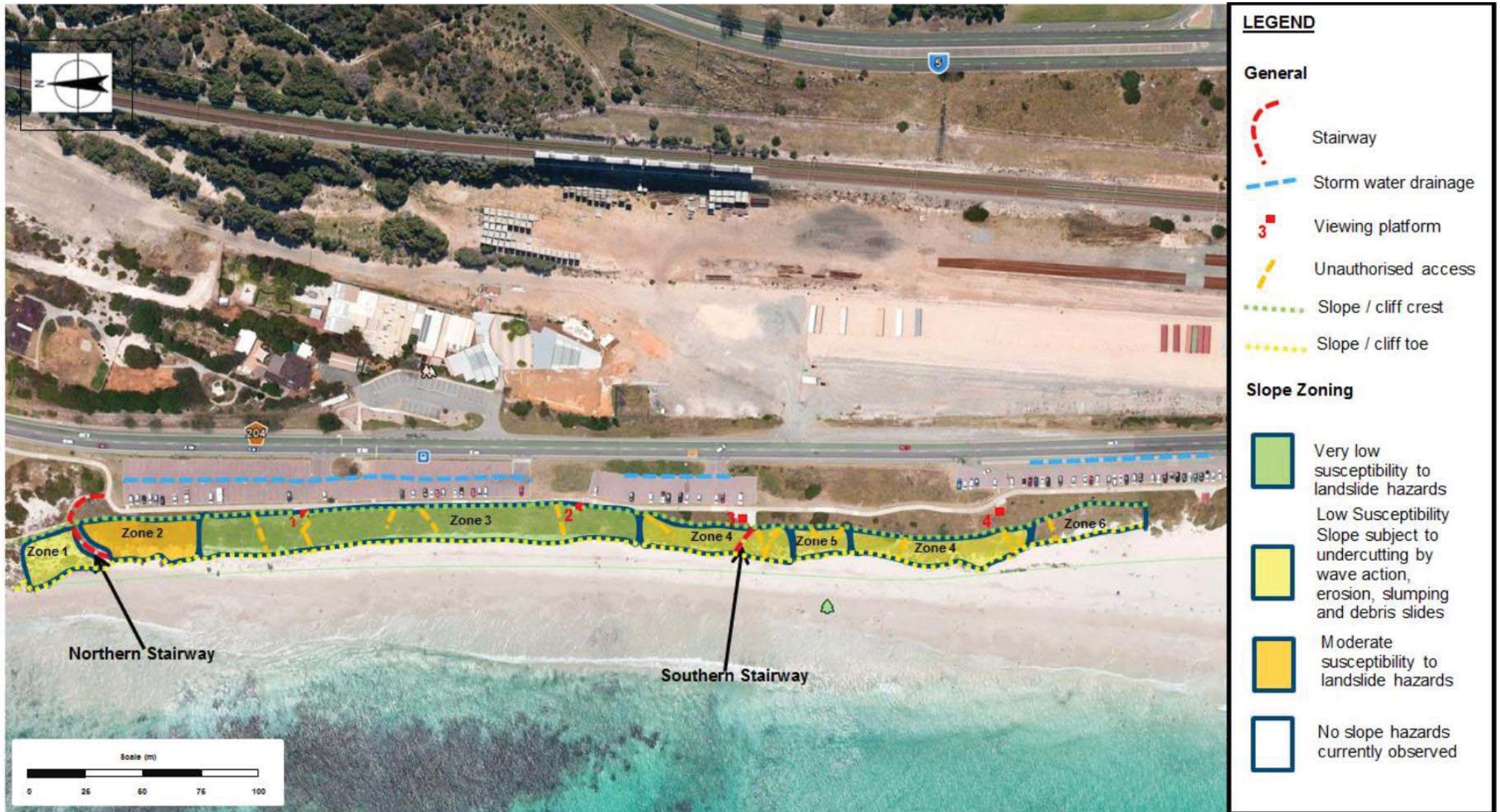
Figure 6 Mosman Park Stability Assessment (GHD 2014).
